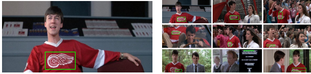
(a) Red Wings logo used as query. (b) Top results of local search
